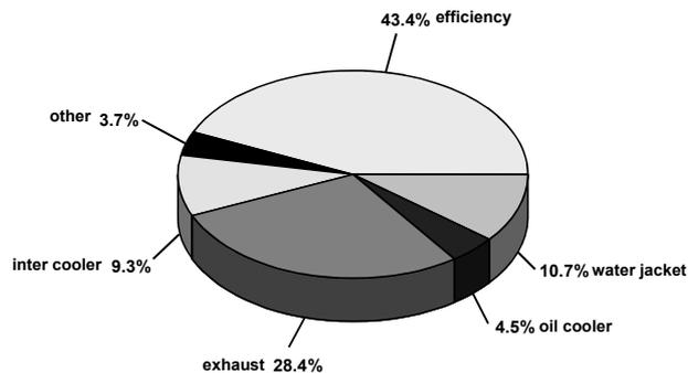
Figure 16: Heat balance of the HEC pilot engine
