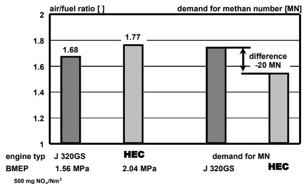
Figure 12: Comparison of Lambda and methane number requirement of Series 3 with the HEC engine
