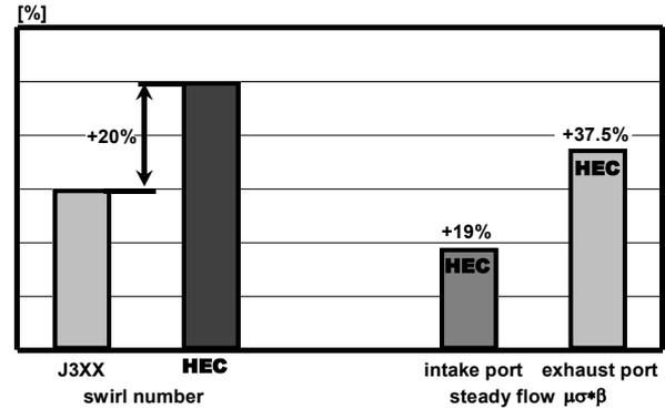
Figure 3: Improvement of the flow coefficients of the 4-valve cylinder head compared with the 2-valve head
