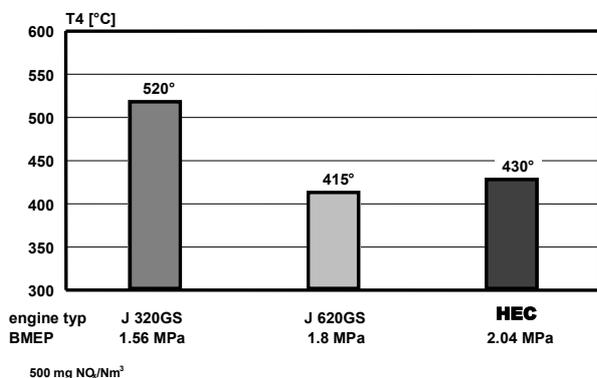
Figure 15: Comparison of exhaust gas temperatures of Series 3 and 6 with the HEC engine
