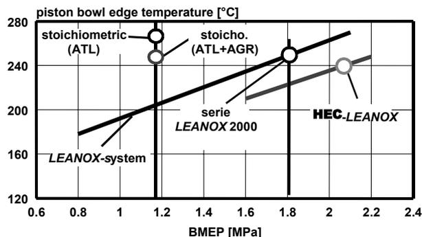
Figure 17: Thermal component stress of various combustion concepts
