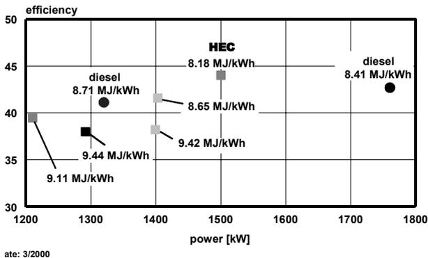
Figure 18: Comparison of the degrees of efficiency (HEC to competition and to modern diesel engines)
