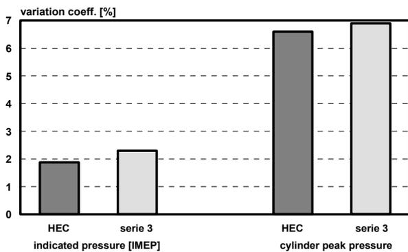
Figure 14: Comparison of the variation coefficient regarding IMEP and peak pressure of Series 3/HEC
