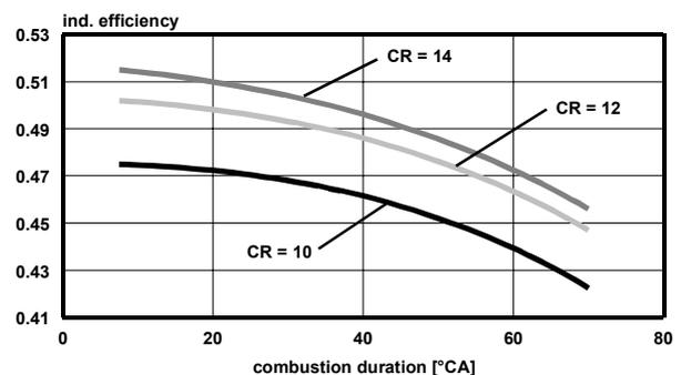
Figure 10: Influence of compression ratio and combustion duration on efficiency
