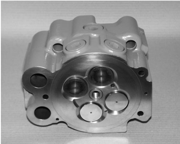
Figure 2: Cylinder head
