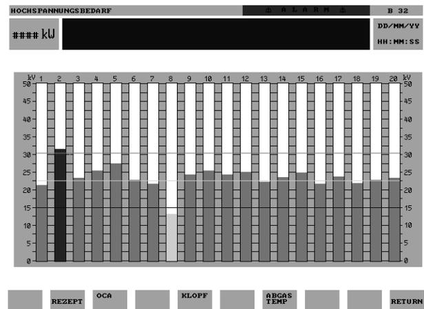
Figure 20: Visualization of actual ignition voltage values on the dia.ne
