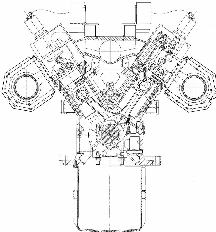
Figure 1: Cross-section of the engine
