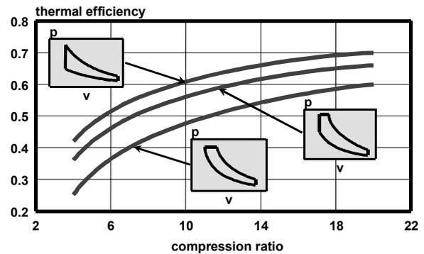
Figure 9: Relationship between compression ratio, type of combustion and degree of efficiency
