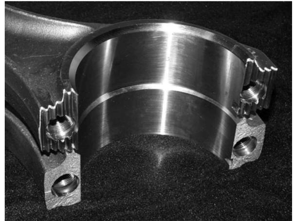
Figure 6: Con-rods produced by means of the crack technology (below) compared with the conventional technology (above)
