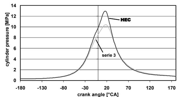
Figure 13: Comparison of the pressure curve at a IMEP of 1.67 MPa Series 3/HEC
