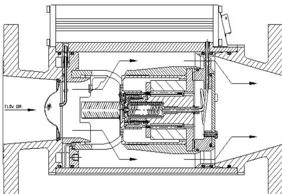
Figure 11: "Tec Jet" gas control valve
