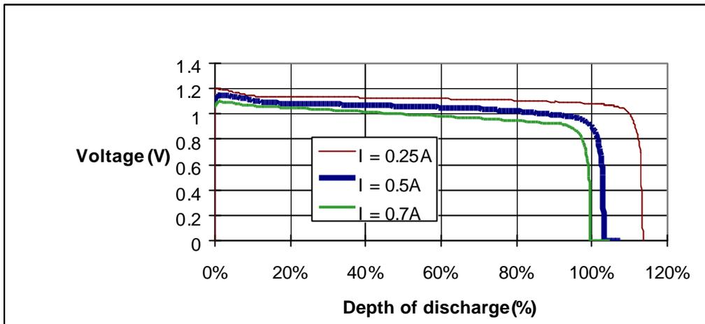
Figure 3. Cell voltages during constant-current discharge, as a function of depth of discharge, for three different current values.
