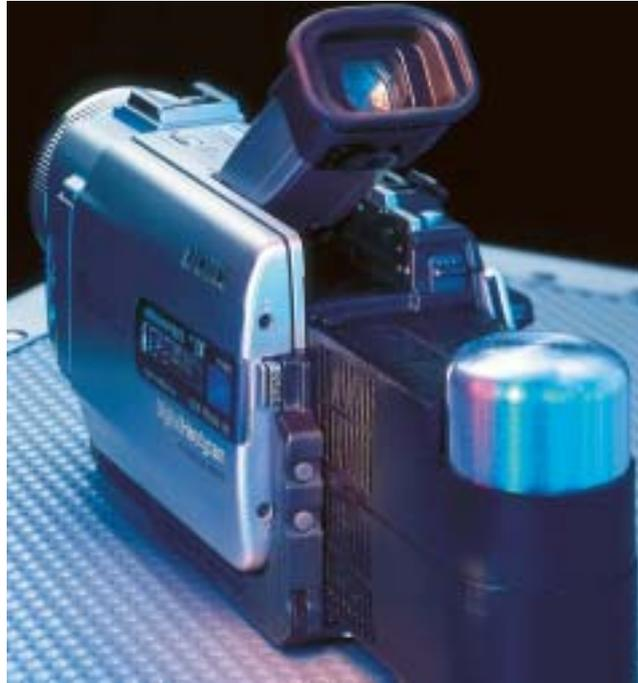
Figure 3: 10 W hydrogen fuel cell system powering a camcorder. This system was developed by the Fraunhofer Initiative Micro Fuel Cell
