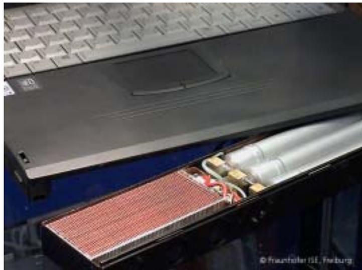
Figure 2: Fully integrated fuel cell system with 50 W peak power, developed by the Fraunhofer Institute for Solar Energy Systems.
