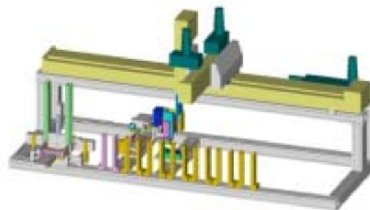
Fig.4b Fully automatized mounting unit for micro-stacks.
