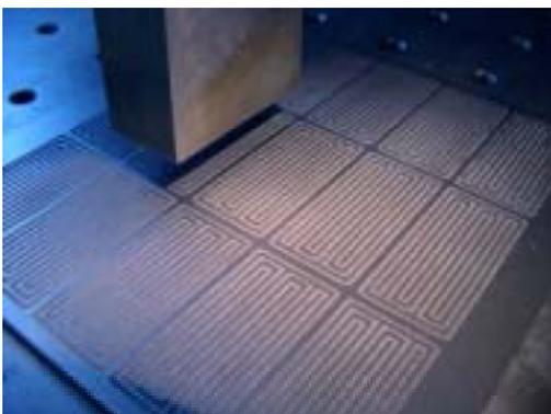
Fig.4a Bipolar plate production by means of ultrasonic machining
