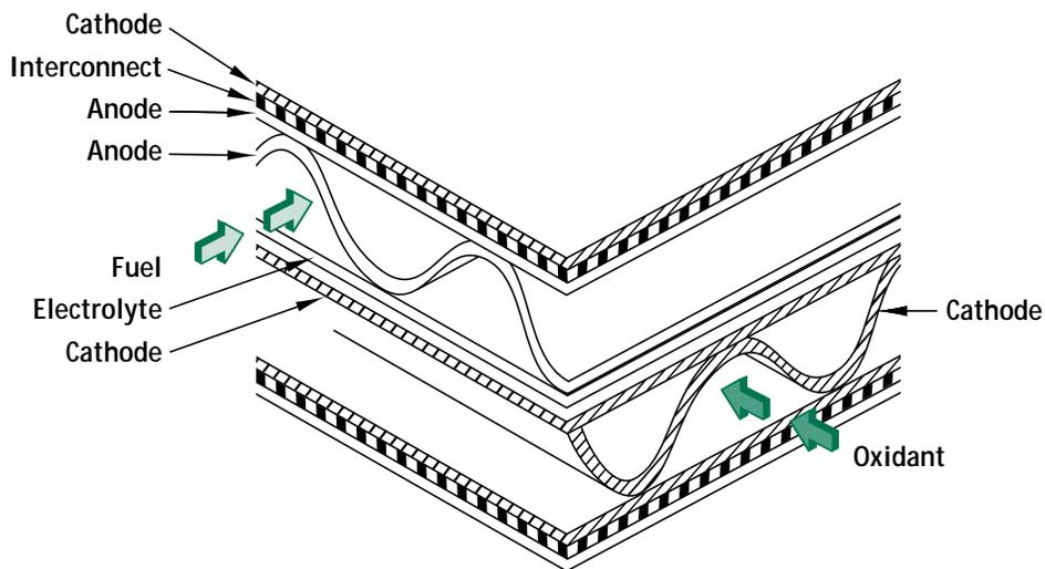
A monolithic solid oxide fuel cell combines three layers of an anode-electrolyte-cathode sequence, with the center layer containing corrugated anodes and cathodes to allow the flow of hydrogen fuel and air. The entire system is sintered into a single ceramic block.
