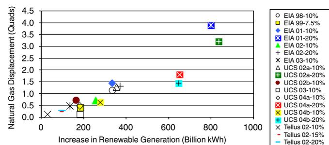
Fig. 1. Forecasted natural gas displacement in 2020.
